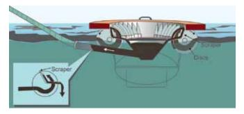
Figures 2 and 3: Small oleophilic disc skimmer, suitable for oils of medium viscosity. Oil adheres to the rotating discs to be scraped off into a sump for pumping to storage. Requires a suitable pump and hydraulic power supply.
