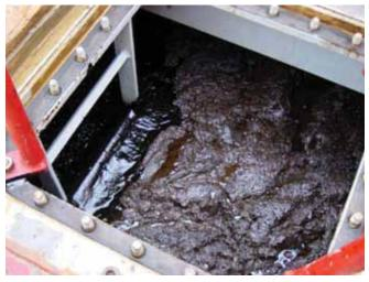
Figure 25: Highly viscous recovered oil in a storage tank on board a recovery vessel (Image courtesy NOFO).
