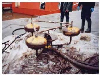
Figure 37: A weir skimmer brought ashore after recovery of heavy oil. Following demobilisation, equipment should be cleaned and overhauled in readiness for future use.
