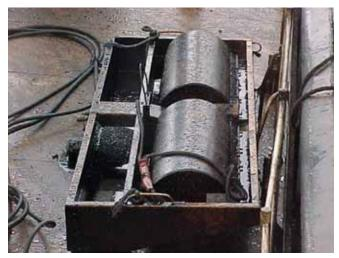
Figure 4: Oleophilic drum skimmer, suitable for oils of medium viscosity. Operates in a similar manner to a disc skimmer in that oil adheres to the rotating drums to be scraped off into a sump for pumping to storage.
