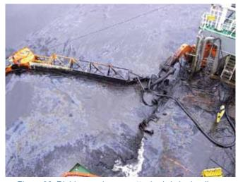
Figure 33: Rigid sweeping arm attached via hydraulic crane to the recovery vessel. The low freeboard and large swell encountered made conditions on deck hazardous for the vessel crew (Image courtesy WSA Cuxhaven).
