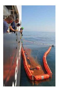
single ship recoverysystem comprising inflatable boom attached to an outrigger and a high capacity free-floating weir skimmer mounted on a Coastguard vessel. The high freeboard allows deployment on the leeside in calmer waters (Image courtesy USCG).
