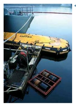
Figure 26: A drum skimmer recovering oil to an inflatable storage barge.
