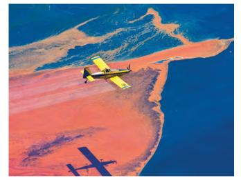
Figure 9: An Air Tractor spraying from an under-wing spray boom onto crude oil spilt from an offshore platform. (Image courtesy of Mark Hamilton Photography).
