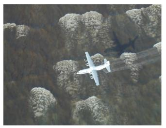
Figure 10: Application of dispersant from a multi-engined aircraft. Here, application in shallow waters was considered beneficial.
