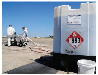
Figure 12: Use of 1m<sup>3</sup> Intermediate Bulk Containers (IBCs) allows straightforward storage and handling of dispersant. (Image courtesy USCG).
