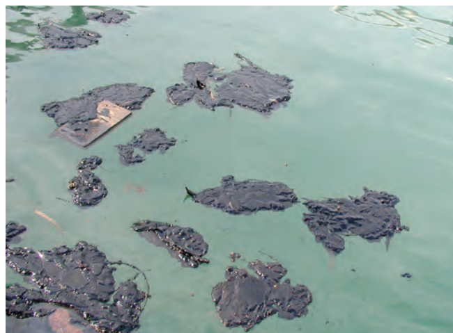
▲ Figure 3: Oils spilled into the sea at temperatures below their pour point form semi-solid fragments. This image shows Nile Blend crude, pour point +33°C, in sea water of 28°C. Such oils are highly persistent and may travel great distances.
