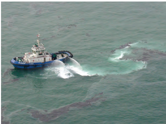
▲ Figure 14: High oil viscosity has resulted in unsuccessful dispersant application, noted by the typical white plume of dispersant around the oil.
