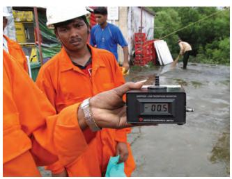
➤ Figure 14: Demonstration of a hand-held phosphine gas monitor outside a hazardous area.
