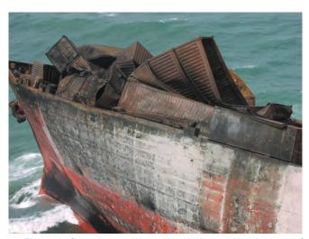
Figure 9: Containers collapsed and distorted by the heat of a fire on the bow section of a stranded Ro-Ro vessel.
