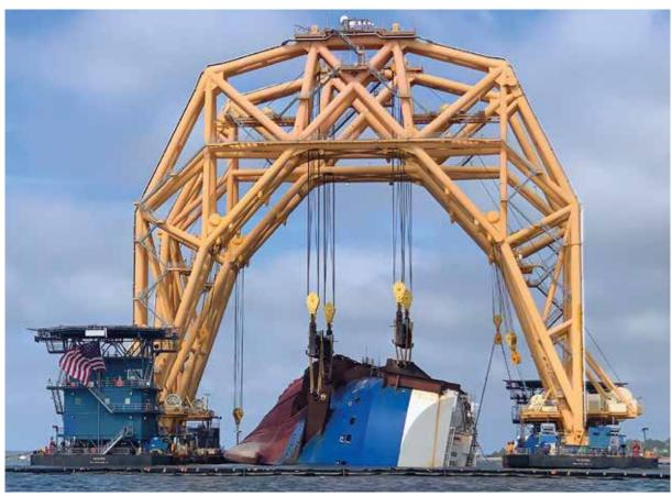
Operations to remove the wreck of a grounded car carrier, USA
