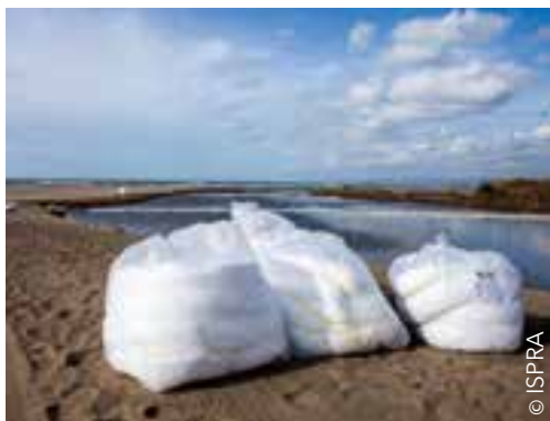
Sorbent booms are used mainly to contain products on the sea surface when used in combination with sorbent sheets or loose sorbents.
