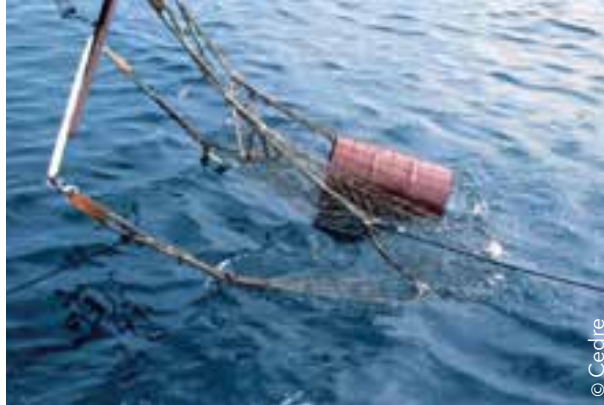
Lifting a drum with a collection net
