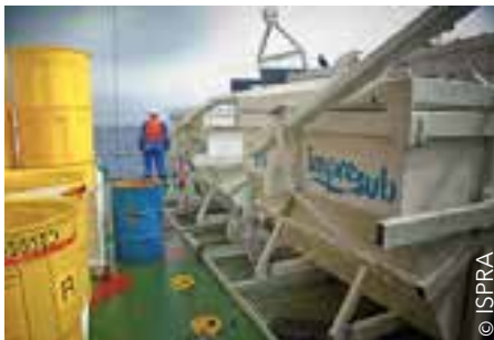
Specific racks and salvage drums realised to collect drums on sea bottom
