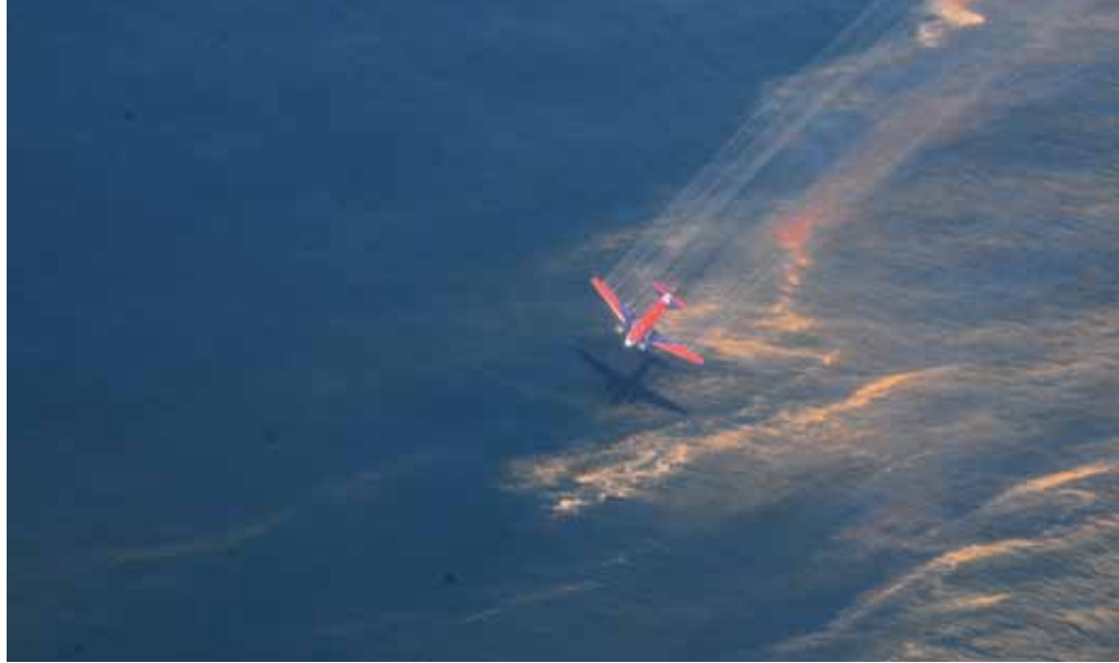
▲ Release of dispersant from a fixed wing aircraft over the DEEPWATER HORIZON oil spill, May 2010 (photo courtesy of USCG)
