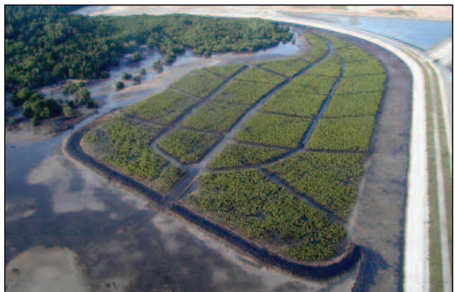
An area of mangrove created from planting individual seedlings in a grid pattern
